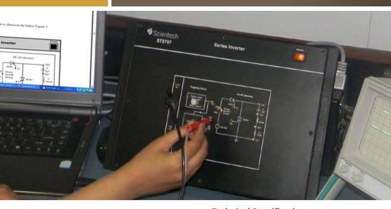
**Scientech 2707** is a platform which is very useful for Students to understand the low voltage application of the SCR in series inverter. 2707 is provided with in built power supply, socket for making different interconnections in the circuit and exhaustive learning material.
