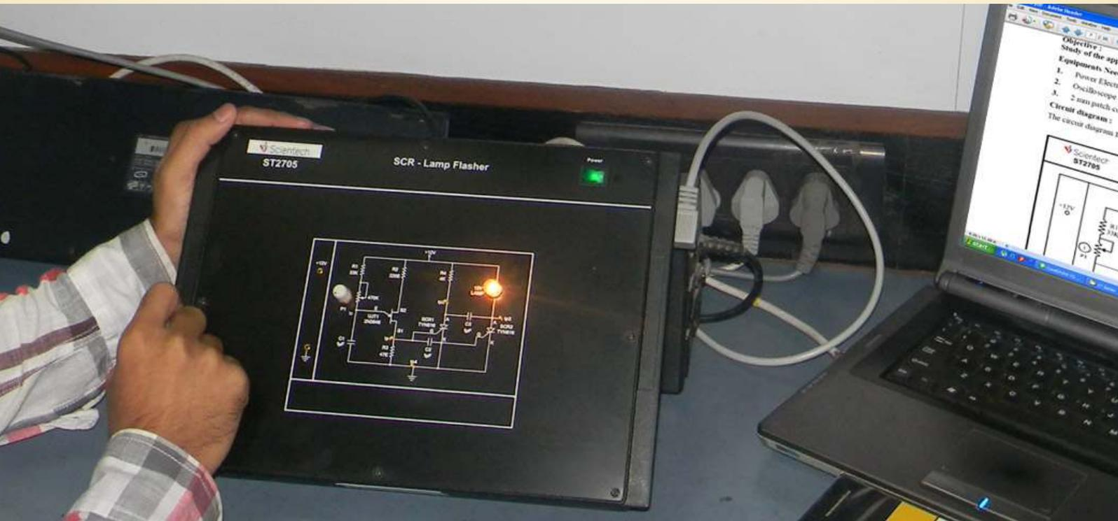
**Sciencetech 2705** is a platform which is very useful for Students to understand the low voltage application of the SCR in lamp flashing. 2705 is provided with the built in power supplies, sockets for making different interconnections in the circuit, and exhaustive learning material.
