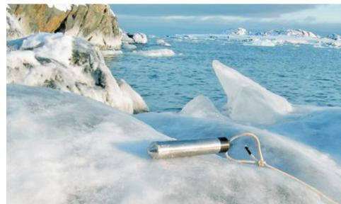
Featuring high accuracy at a great price and ease-of-use, with no cumbersome vent tubes or desiccants to maintain, this logger is ideal for recording water level and temperature up to 30-ft depths in shallow wells, streams, lakes, freshwater wetlands (stainless-steel), saltwater/brackish wetlands and tidal areas (titanium).
