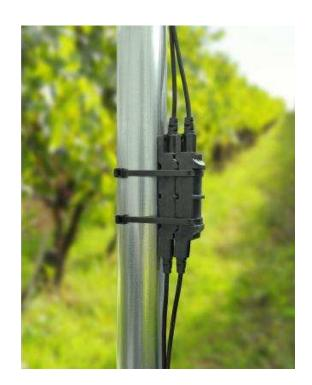
A temperature/relative humidity sensor designed to work with all HOBO data loggers that accept Smart Sensors. All sensor parameters are stored inside the Smart Sensor, which automatically communicates configuration data information to the logger without any programming, calibration, or extensive user setup.
