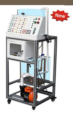
Scientech 2421R Water Level Control Rig with PLC enables students and practicing engineers to gain invaluable practical experience on the principles and application of programmable logic controllers. The objective is to connect and program programmable logic controller to monitor and control the level of water in a tank system. Scientech 2421R consists of a Delta PLC, float switch, solenoid valve, polycarbonate sump tank, measuring tank, water pump, start, stop pushbutton, and its indicator.
