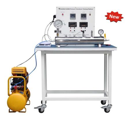
**Scientech 2308M Pressure Transducers Test Bench** is designed to explain concept of pressure measurement. It helps students & industry professionals to understand operation of pressure transducers in detail. Scientech 2308M Pressure transducer training platform includes different types of pressure sensors including capacitive pressure transducer, load cell, bourdon tube pressure gauge, and pressure vessel.
