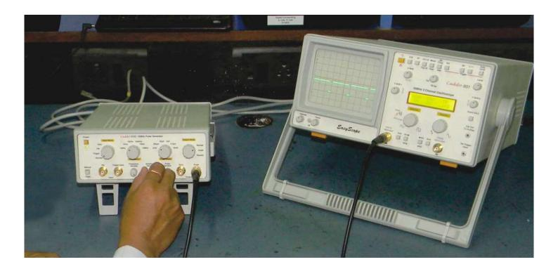
Scientech 4066 Pulse Generator offers low rise and fall time pulse signals at high repetition rate up to 10MHz to meet today's Test & Measurement needs. The Scientech 4066 features pulse width controls in 6 steps with variable adjustment. It's External and Manual Triggering, FM and Gating output is very useful in Education & Training. Simultaneously Pulse & Sync outputs can be utilized for various applications in Electronic Laboratory, R&D & Industry.
